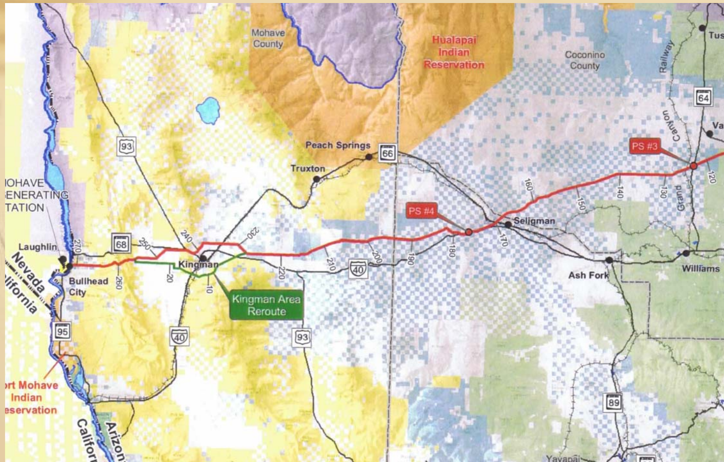
Black Mesa Complex – coal slurry pipeline alignment
