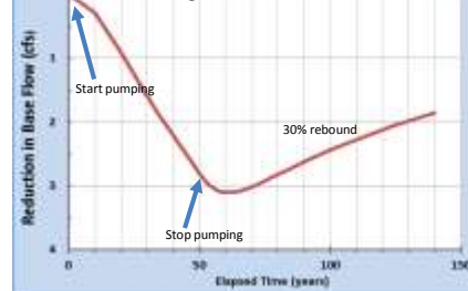
Calculated Reduction and Recovery of Base Flow at Paulden Gauge with 12,000 ac-ft/yr of Pumping at the Big Chino Water Ranch
