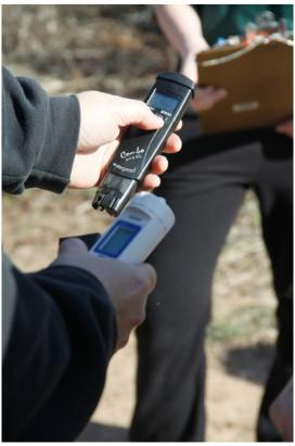
Figure 29. The Hanna combo tester Photo credit: Mark Coryell
