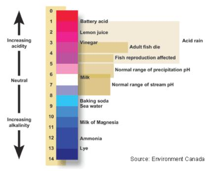
Figure 28. The pH scale Source: Environment Canada
