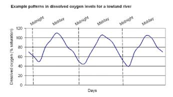
Figure 26. Example patterns in dissolved oxygen levels for a lowland river Source: New Zealand Ministry of the Environment website<sup>43</sup>
