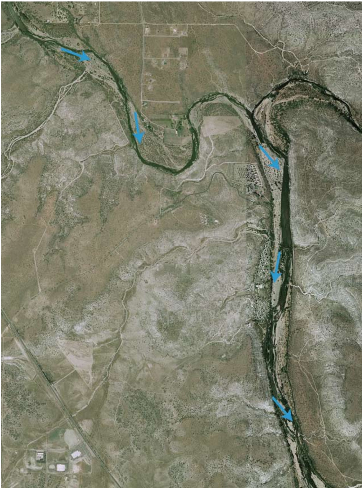
Figure 3-5. Gravel bars of alternating orientation deposited in the flood channel form the architecture of the system through which the low-flow channel flows. Low-flow riffles typically exist at the upper ends of large gravel bars, and pools typically are formed below the downstream ends of the large gravel bars. Blue arrows show several large gravel bars and their general orientation. The confluence with Oak Creek is in the upper right part of this figure.
