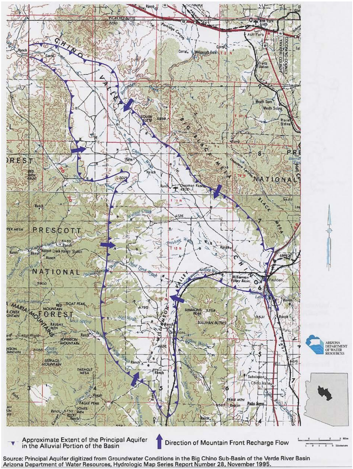
Figure 9.1. Principal aquifer in the alluvial portion of the Big Chino Sub-basin (ADWR, 2000, Figure 4.3).
