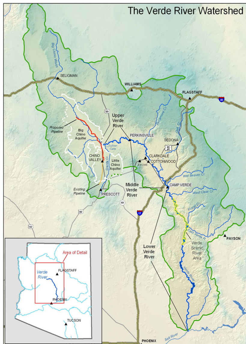
Figure 19. Location of planned groundwater transfer pipeline.
